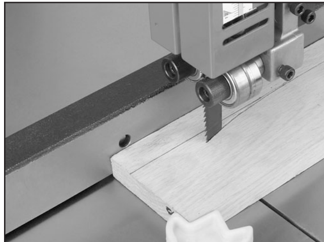
Figure 41. Blade leading away from line of cut.
